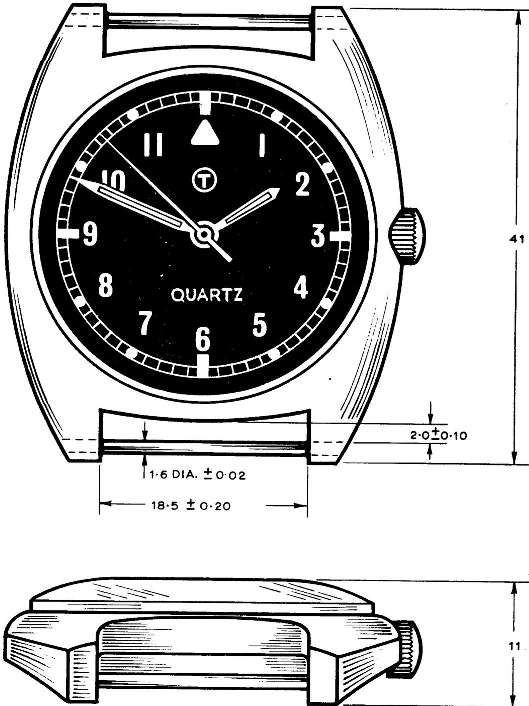
BATONS AT 3,6,9 AND 12 TO BE LUMINIZED 2 MILLIMETRES BY 1 MILLIMETRE.
